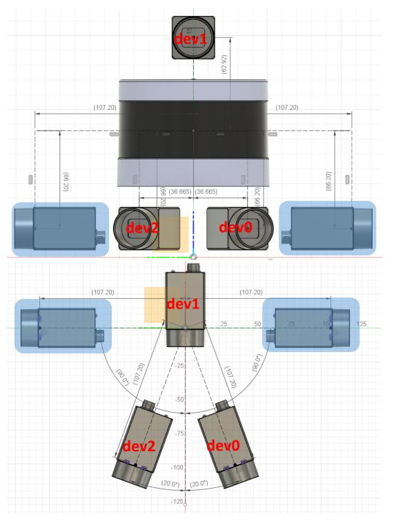
The cameras marked with blue on the diagram below are unavailable for the competition.
