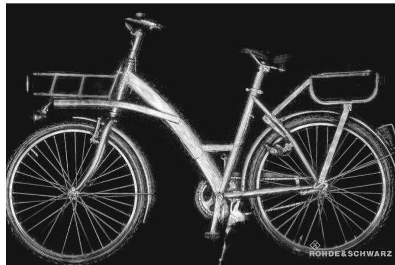
mmWave picture taken by Rohde&Schwarz, frequency 70 GHz to 80 GHz, several thousand transmitting and receiving antennas
